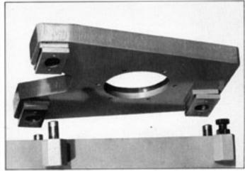
Bolsters are provided with three ground locating plates which fit exactly on three hardened pegs. They are secured by clamping plates with screws tightened from the upper surface. With the bolster in place and the screws loosened, the tools can be aligned and after the screws have been re-tightened the bolster can be lifted off and replaced repeatedly in perfect alignment. The fourth corner rests on an adjustable screw to prevent rocking.
