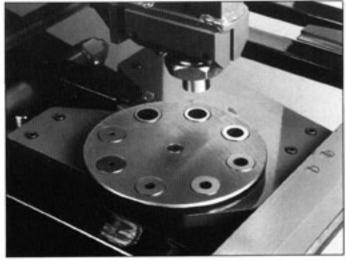
Where regular punching of different size holes up to 18mm dia is carried out, a special Bolster and Turret assembly is available, which enables rapid changeover from one hole size to another.
