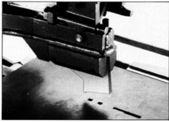
Two knurled Stop Screws control the depth of entry of blades and punches into the dies. The block on which the longer screw abuts is pivoted so that it can be swung in or out of use instantly. The setting illustrated is typical for making a small slot where only the top of the blade is required to enter the work, which is then turned and the slot completed from the other end.
