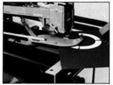
Circumferences finish as a series of short flats and this is generally acceptable without further work, as the out-ofround, using a 25 x 6mm blade, is only 0.5mm at 300mm dia. This is a quick way to cut out large holes and discs to about 800mm dia and in up to 3.2mm mild steel. Radial slots are also simple to achieve.
