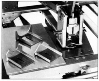
A selection of stripper feet for round or square punches is also available for up to 75mm dia holes.
