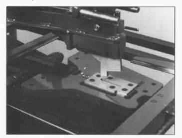
Each machine is fitted as standard with a 50 x 6mm heeled blade and 4 piece adjustable die on type 'A' Bolster. One stroke cuts a slot 50 x 6mm in up to 3.2mm thick mild steel. Longer slots are cut by successive strokes and shorter ones by using the Stop Screws as illustrated on page 5. Shorter and thinner blades are also available.
