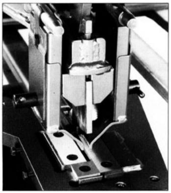
All machines are supplied with a pair of stripper main plate assemblies fitted with stripper feet for flat blades.
