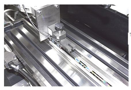
The Heidenhain VLM scale during inspectio for positioning and repeatability.
