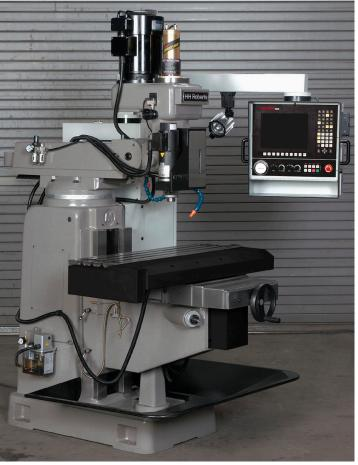
Above is our new compact version with a 42" table, the X axis motor in front of the table and protected by the black guard. This saves about 30" of floor space left to right.
