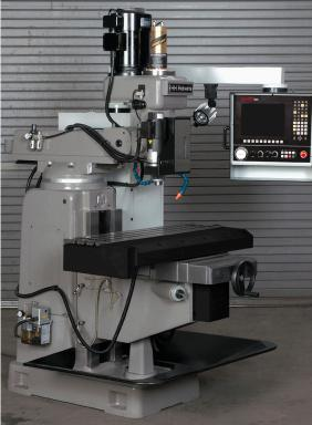
Above is our new compact version with a 42" table, the X axis motor in front of the table and protected by the black guard. This saves about 30" of floor space left to right. (This photo is actually a 4-GL model)
