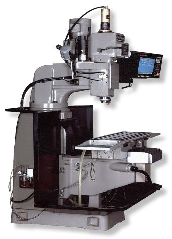
This version has a saddle almost as wide as the table. The X and Y axis ballscrews are mounted like those in a machining center, avoiding the problems associalted with the Y axis nut housing in typical turret mills with handwheels.
