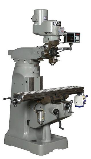
This is the manual version. A photo of the machine with the CNC fitted is not available at the time of printing. This machine can also be fitted with the gearless vector drive head as on the machines on following pages, This gives spindle control on the CNC for speed settings, automatic start and stop and tapping.
