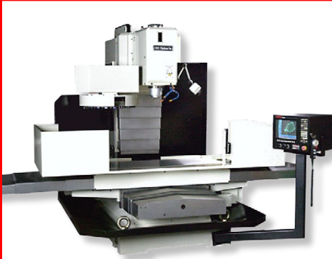
Vertical bed mills with machining center heads to 31" x 20" to 60" x 32"
