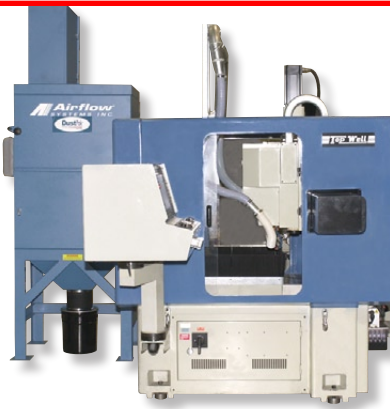
Bridge type electrode and engraving mills with 25,000 rpm spindles.
