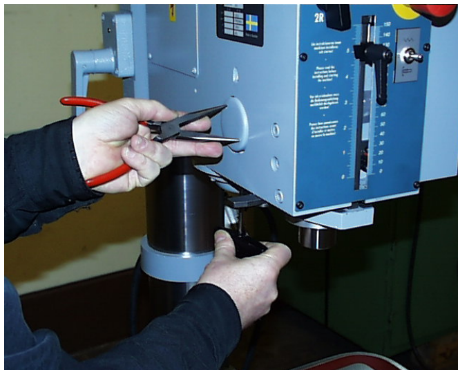
Picture 5: Removing the spring case
