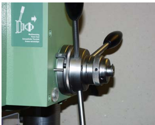
Picture 2. Inserted coupling
