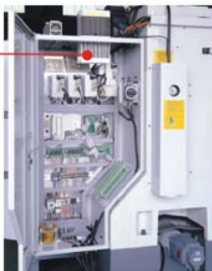
NC Electro-Control Box
