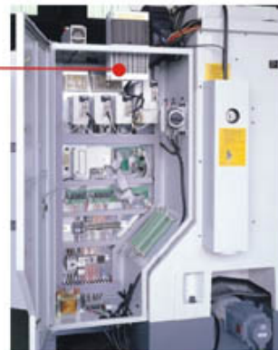
NC Electro-Control Box
