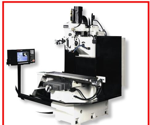
Bed mills with gearless quill heads to 7 1/2 Hp and handwheels.
