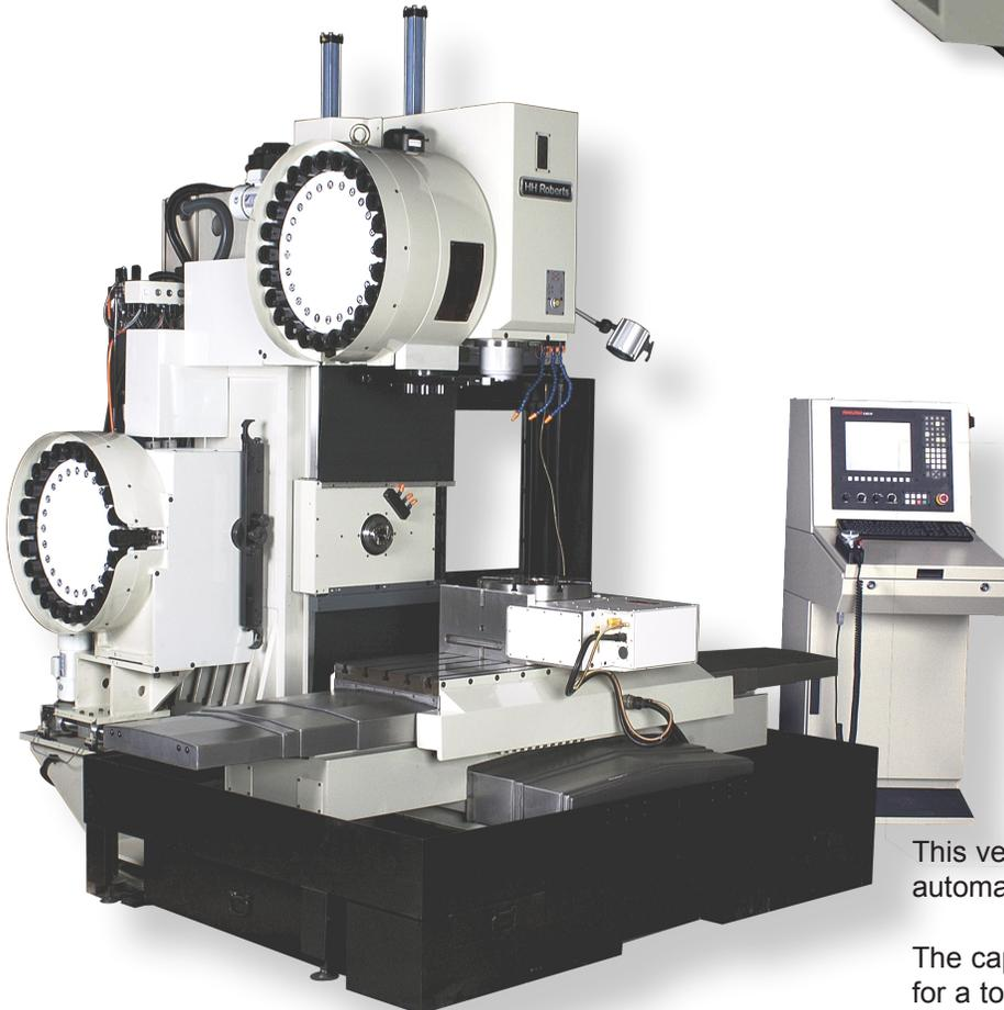
This version of the H/V has TWIN 24 tool arm type automatic tool changers fitted, for a total of 48 tools.
