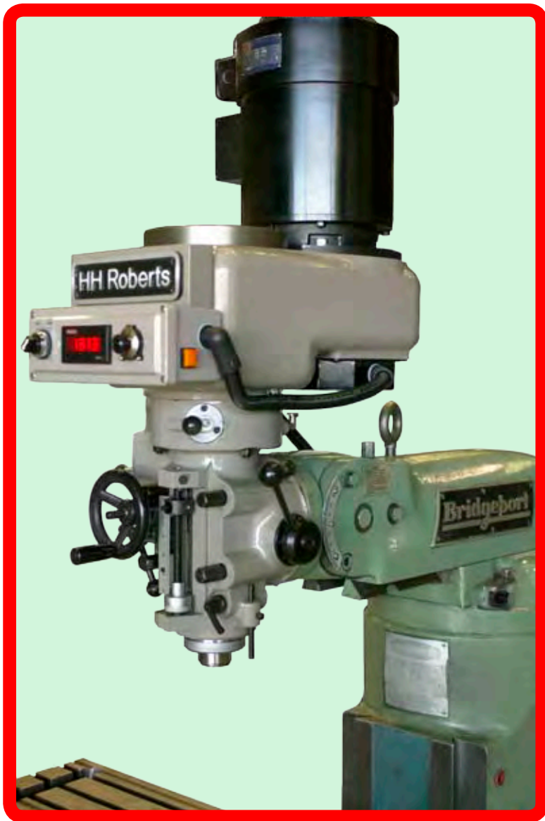
The standard R-8 head mounted on an old Bridgeport.
