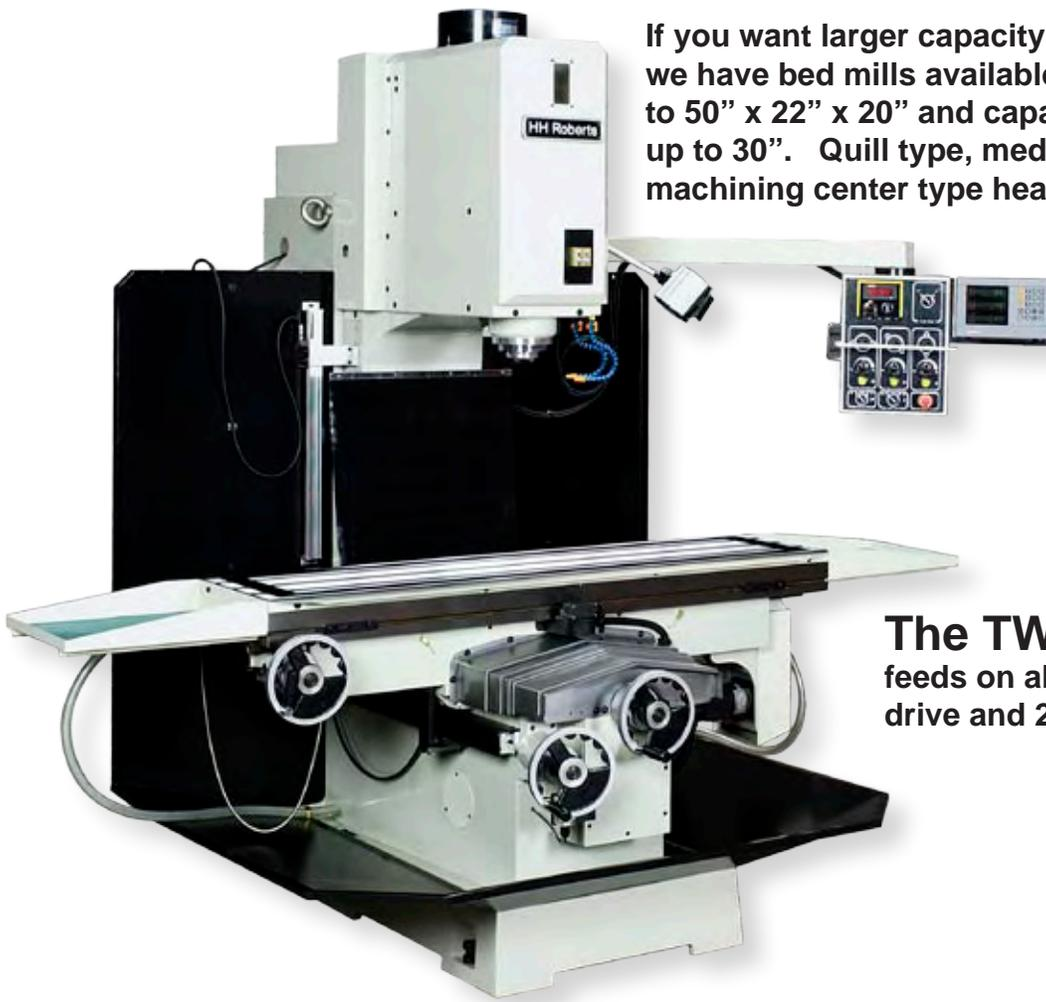
**The TW-50-RH** with servo feeds on all 3 axes, 15 Hp spindle drive and 2,000 lb table load.
