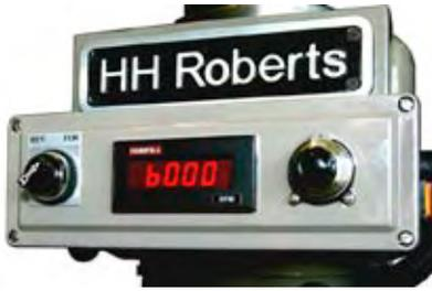
The heart of our GL knee mills is our vector drive heads. With about 85 less parts than a Bridgeport vari-disc type head, maintenance is reduced to near zero. Only 3 moving parts in the drive train. The motor shaft and pulley, the drive belt, and the spindle and pulley. Gone are vari-disks, springs, brake pads and fingers, hi-lo clutch and shift mechanism, back gears and the extra timing belt, speed adjusting handwheel with its inaccurate setting, chain linkage etc.
